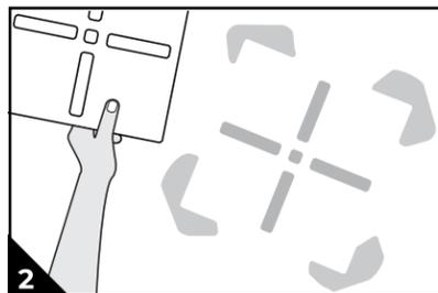
2 Remove AeroStencil and allow paint to dry.
