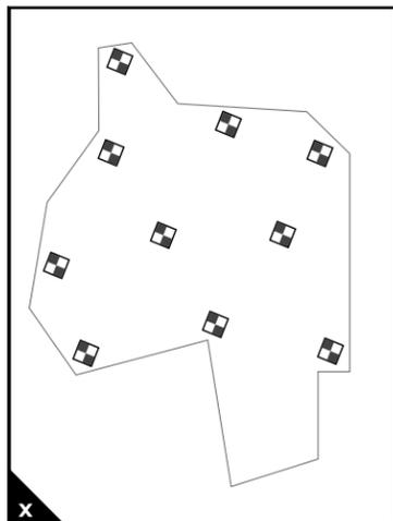
Fail: AeroPoints are missing from one part of the site (protruding area at bottom).
