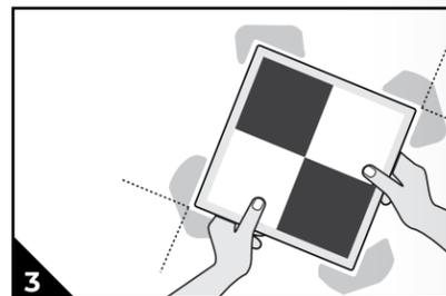
3 Place AeroPoint on top of AeroStencil mark, using painted corners to align exactly. Activate each AeroPoint and complete flight as usual.
